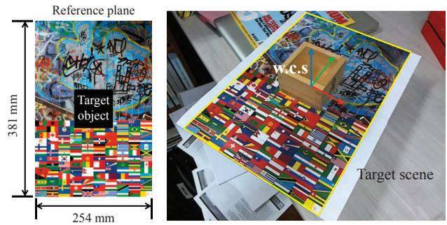
Fig. 8. Setup for the comparison of 6DOF camera poses. **Left**: Reference plane, **Right**: Target scene and 3D object.
